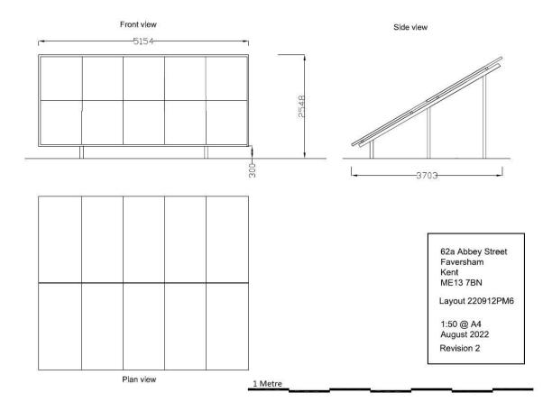
Figure 1. Proposed installation with vertical uprights on horizontal 'sledge'- see Figure 2
