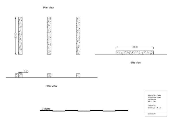
Figure 2. Ground 'sledge' for solar panels
